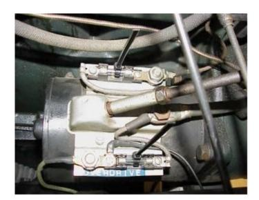
This particular Model A has a second fuse circuit to accommodate a Borg Warner overdrive. The zip ties around the fuses are to provide a means to easily remove the fuses when the car is not in use.
