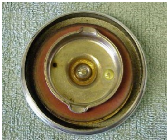
Modified gas cap with a small rivet epoxied into place opposite from the vent hole.
