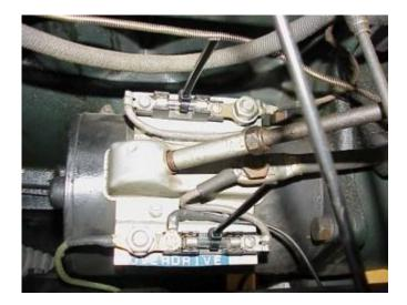
This particular Model A has a second fuse circuit to accommodate a Borg Warner overdrive.
