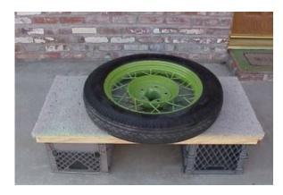
The wheel is placed on the board with the hubcap facing down into the 9" hole. To make the tire slide on the rim easy obtain a large can of baby powder. Liberally sprinkle the powder on the inside of the tire and especially around the bead. Coat the inner tube with powder as well.
