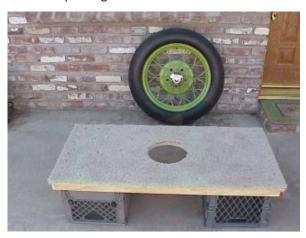
The board is made of 3\4" plywood 44" long and 21" wide. There is a boarder 1&1\2" wide nailed around the bottom edge. Two plastic "milk carton" containers fit nicely under the board and will easily support my weight along with the wheel and tire. A 9" hole is cut in the center and the surface is covered with carpeting.
