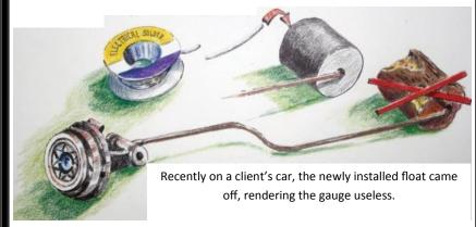
After 15 minutes of fishing for it in the tank, I groped for a simple cure. Although it adds a bit of weight, I gently forced a two-inch piece of solder into the float, along-side the already installed arm. Common, thin electrical solder offers a nice, snug fit.
