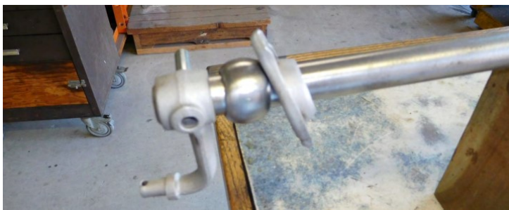
Shown in the photo is one end of the shaft showing how the lever mounts to the shaft. A tapered pin is driven into the hole in the lever and shaft. A new pin can be seen protruding from the far side of the lever. The frame hole is beveled on one side to provide half of the bearing race. The bracket on the right is the other half of the bearing race, and bolts to the frame with two mounting bolts. The other end of the shaft has the same assembly, except the two levers are a left and a right. When installed each must point outward toward the rear of the car. On the bottom of each lever is where the E-brake rods that attach to the brake levers on the rear backing plates attach.
