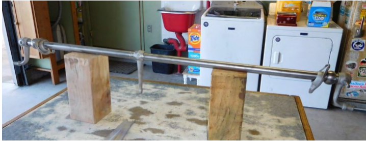
This photo shows the later E-brake cross shaft removed from a 1930 Tudor. Each end of the shaft protrudes through a hole in the frame on each side. The hole is beveled on the inside of the frame in the shape of the bearing and provides one half of the bearing race.
