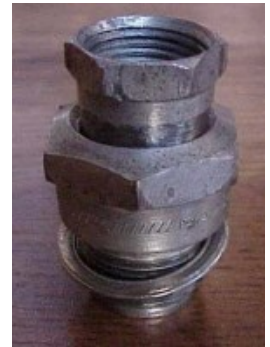
The modified base of a 3X spark plug and the adapter attached with 1/2"-20 threads.
